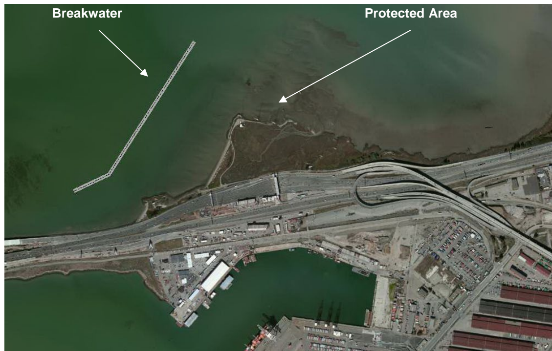
Figure VII: A potential breakwater placement and configuration offshore of Radio Beach that will minimize wave action and overtopping of the levee as sea level rises
