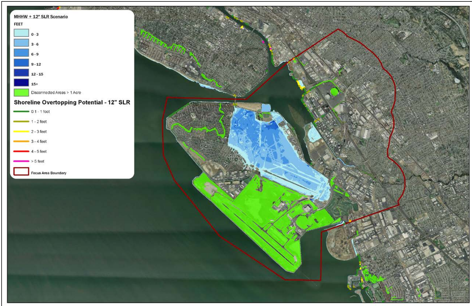
Figure 1. Initial Inundation Maps Showing Inundation of Bay Farm Island with 12 inches of SLR
