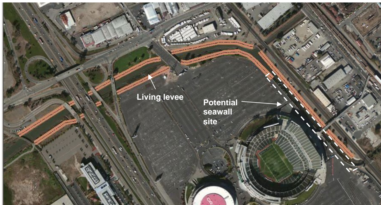
Figure VIII: The layout and footprint of the living levee (brown) and the section where seawall might be necessary due to space limitations
