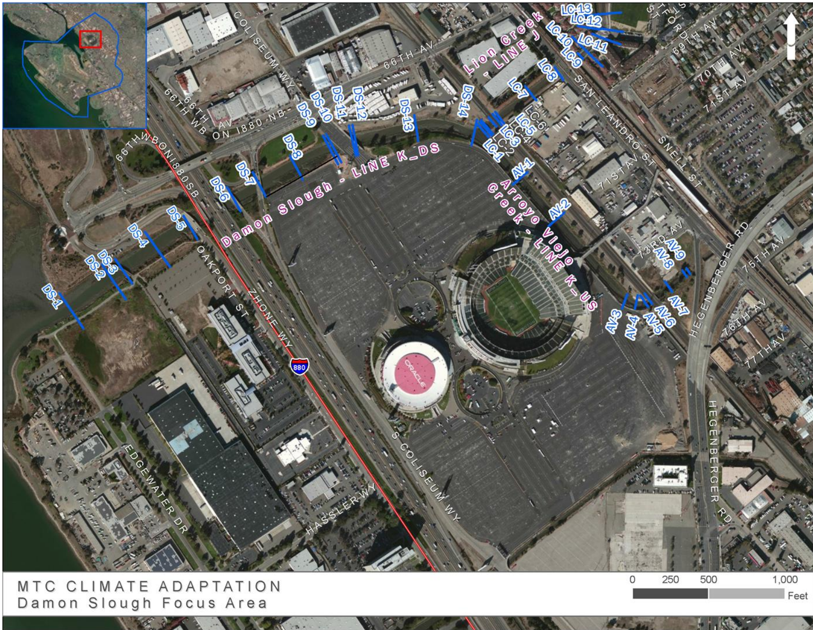
Figure 3: Locations of Modeled HEC-RAS Cross Sections
