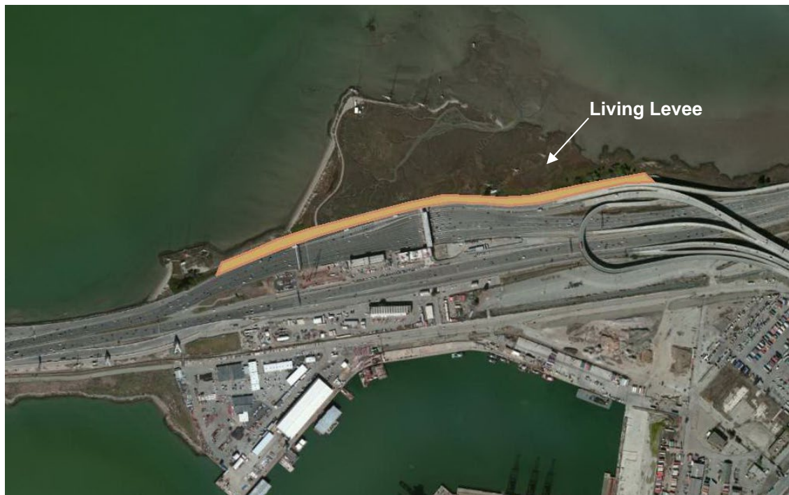
Figure VI: Approximate footprint of the living levee designed to protect I-80 from at least mid-century sea level rise with a 100-year total water level
