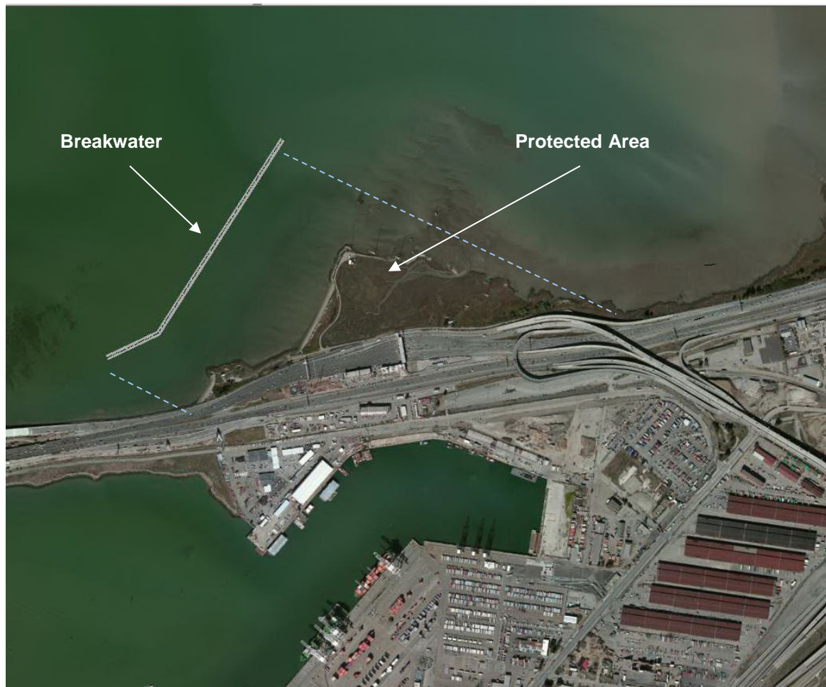
Figure 5-13: A potential breakwater placement and configuration offshore of Radio Beach that will minimize wave action and overtopping with 36 inches of SLR. The protected area where the wave heights will be reduced by at least half due to diffraction is shown within the dotted lines.
