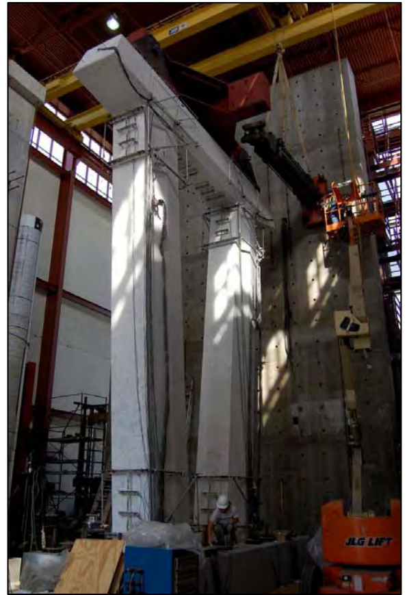
Mock-up of Dumbarton Pier Columns Undergoing Seismic Testing
