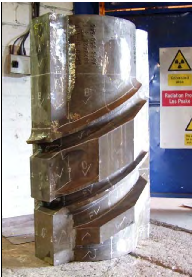
Trial Cable Band Assembly
