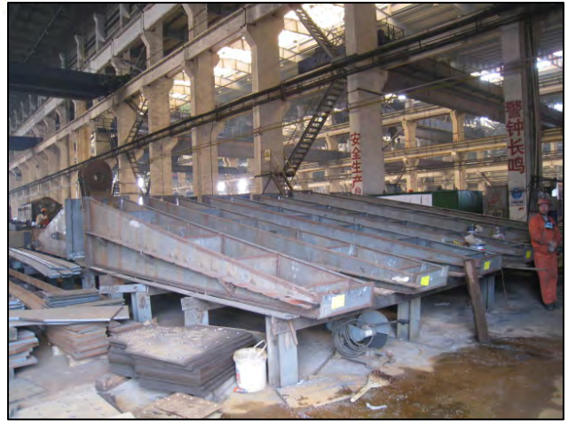
Bike Path Bracket Assembly in Bay 5
