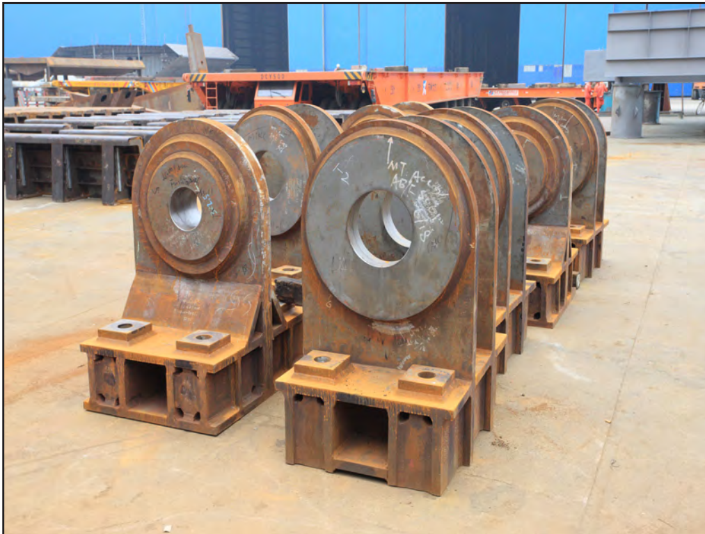
Self-Anchored Suspension Bridge Lifting Attachments for the Roadway Boxes
