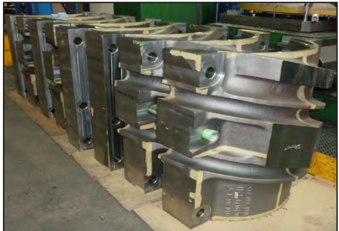
Cable Bands Ready for Painting
