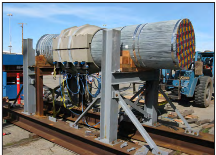
Sample of Cable Band Compaction Testing Performed at Pier 7 in Oakland
