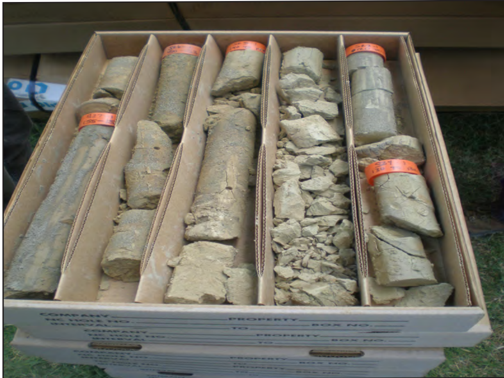
Antioch Bridge - Soil Samples from Seismic Monitoring Down Hole
