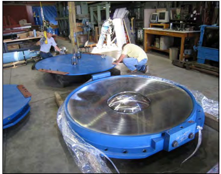
Prototype of Bearing for the Antioch Bridge Seismic Retrofit Project
