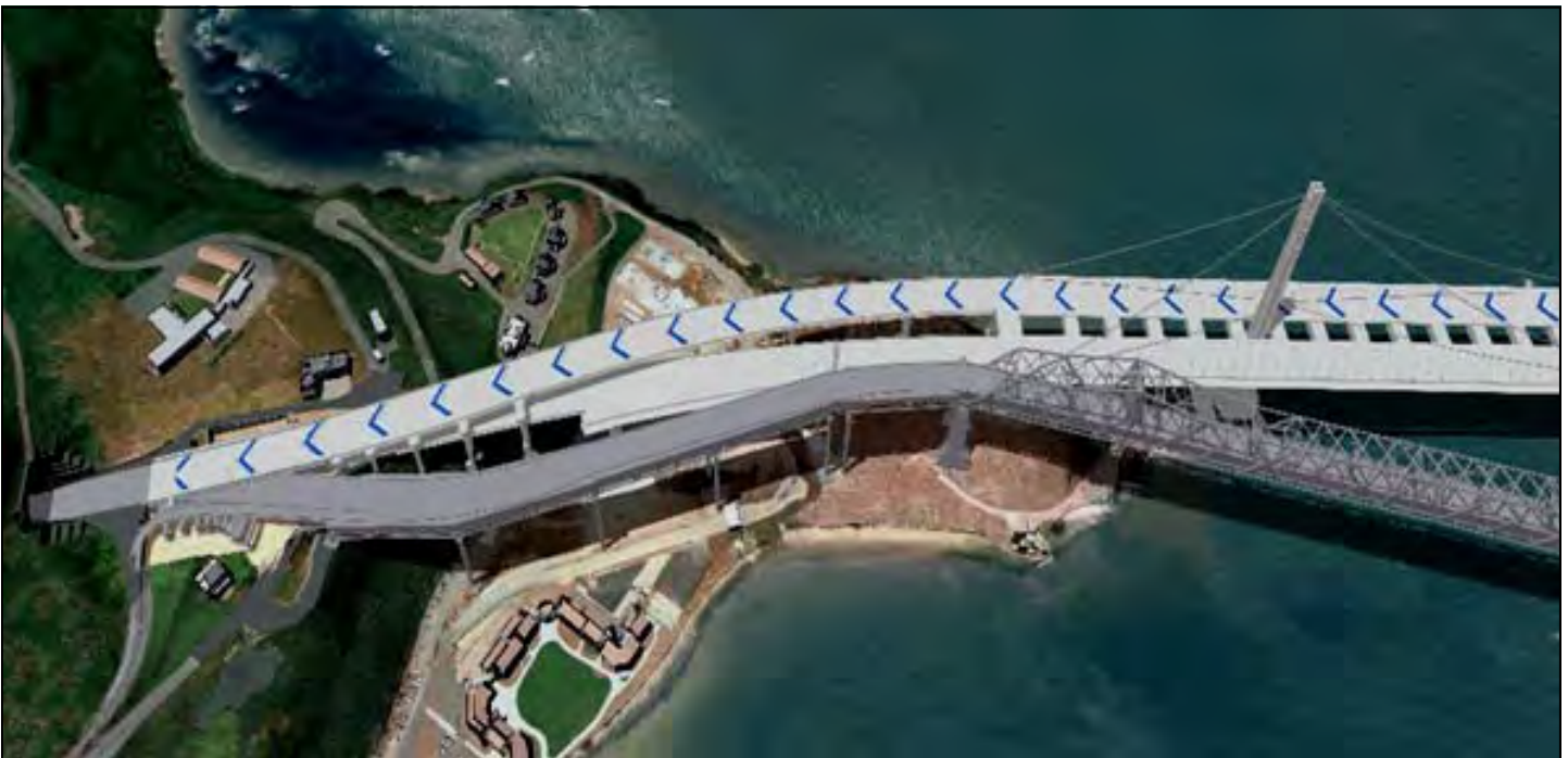
Rendering of Future Yerba Buena Island Transition Structures (top) with Detour Viaduct (bottom)
