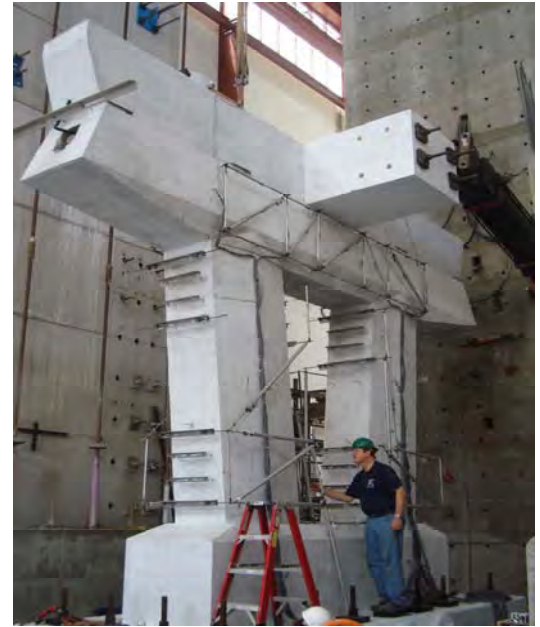
Mock-Up of Dumbarton Pier Columns Undergoing Seismic Testing
