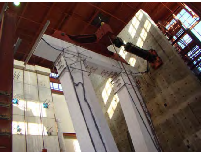
Dumbarton/Antioch Bridges Mock-Up of Dumbarton Pier Columns Undergoing Seismic Testing
