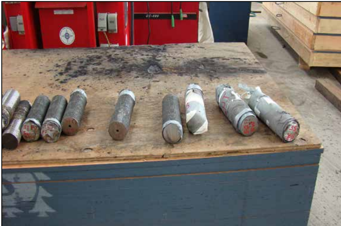
Trimmed E2 Shear Key Anchor Rods
