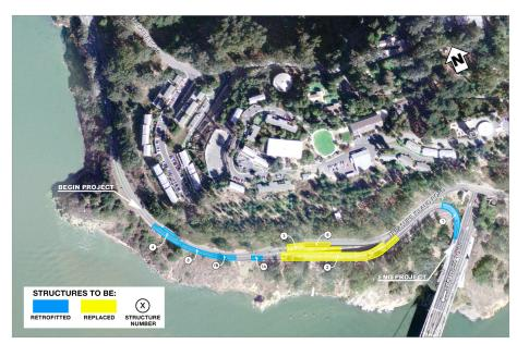
The YBI West-Side Bridges Retrofit project will retrofit eight existing bridge structures along Treasure Island Road to meet current seismic safety standards. Five of the structures (shown in blue) will be seismically retrofitted, while three (shown in yellow) will be demolished and replaced.
