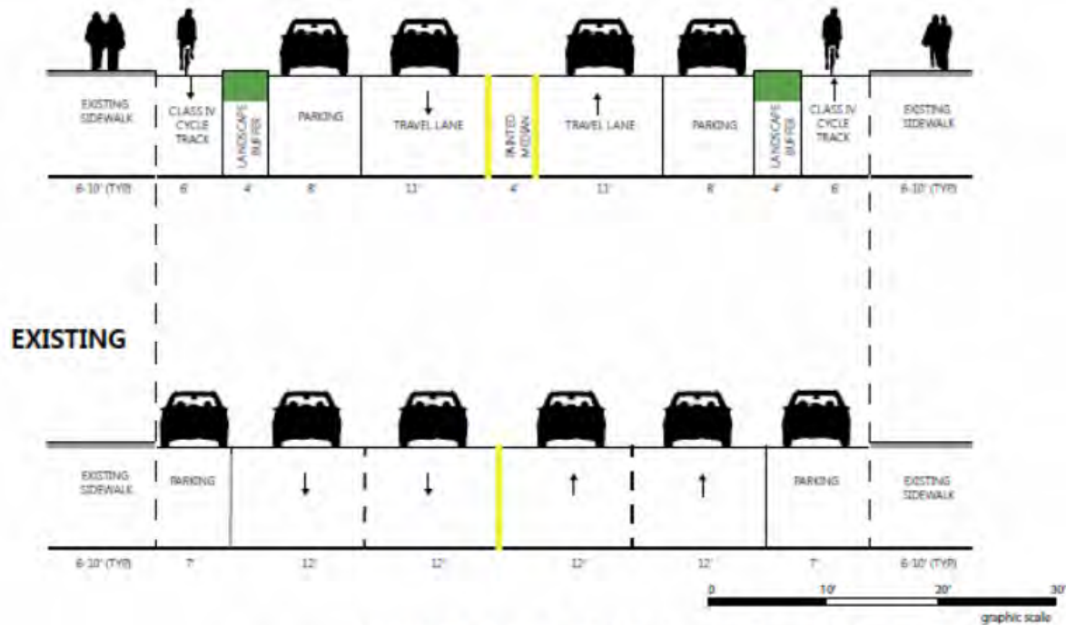
MARKET AVENUE TO SOUTHERN CITY LIMIT CROSS-SECTION RUMRILL BOULEVARD CYCLE TRACK & PEDESTRIAN IMPROVEMENTS
